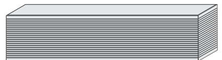
127 layer HSHT Filled Beam: (not to scale) 2 layers Nylon, 125 layers HSHT Glass CFF: Heat Deflection: 150 °C
